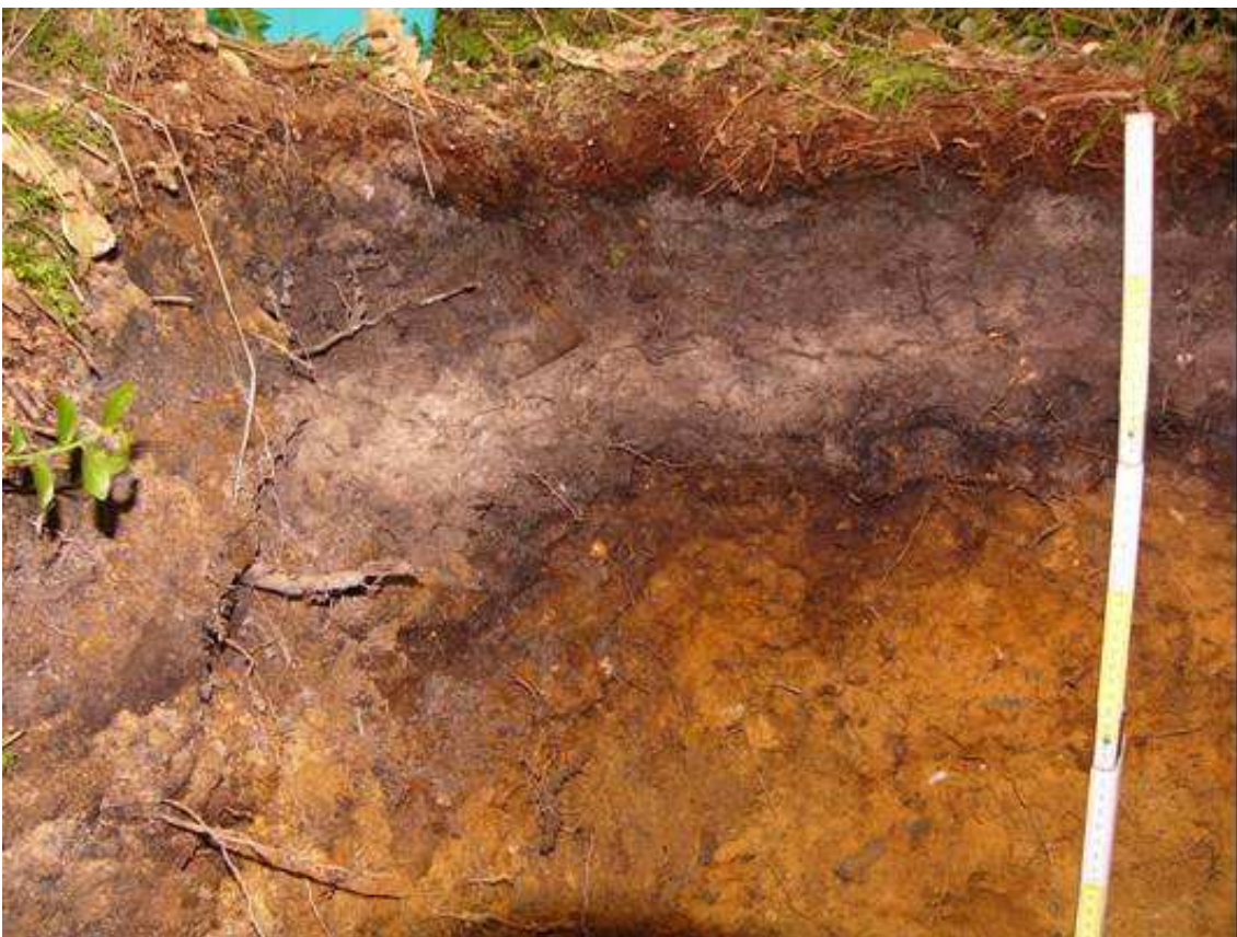
Photo 32: View on the back side of profile 703. At this level the eluvial horizon (H3b) is well developed (Photo by JM)
