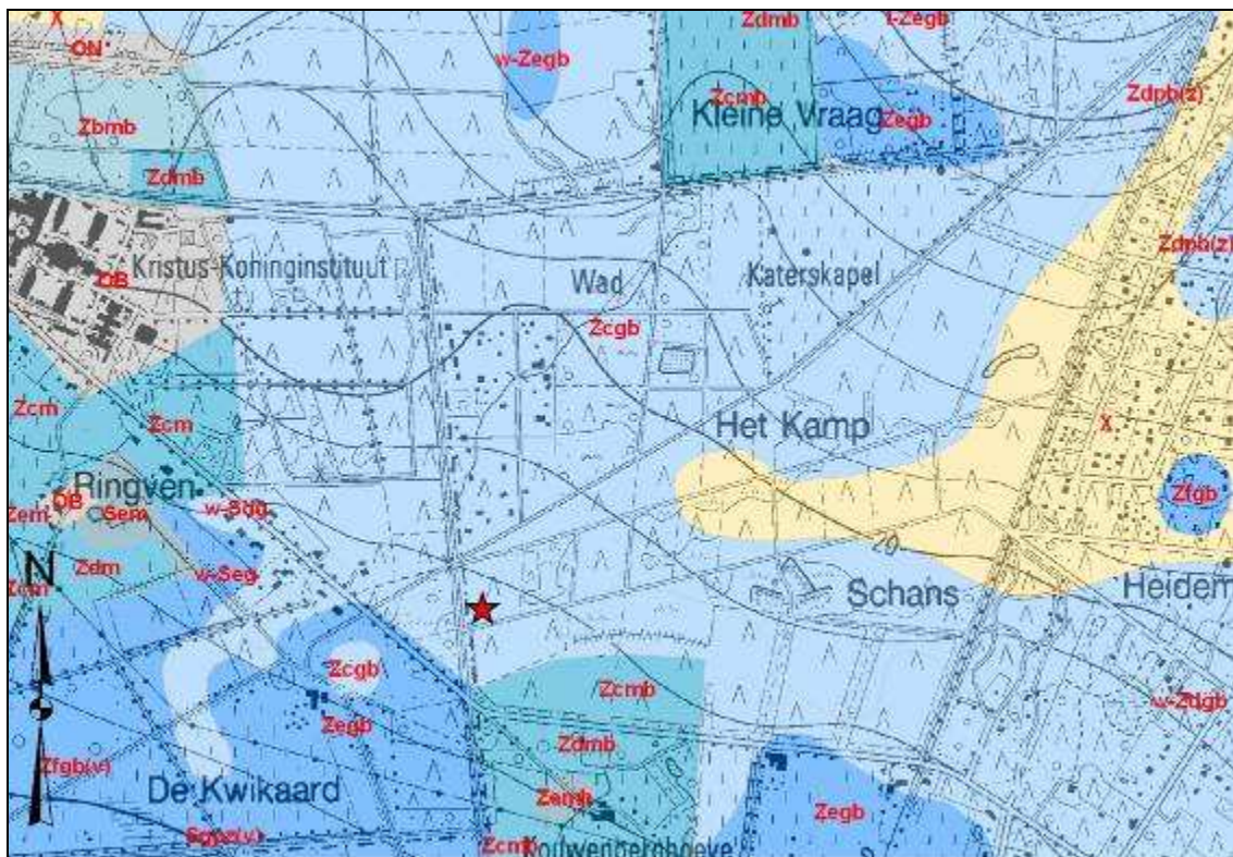
Figure 23: Soil map of the surroundings of P505, Schilde. The sandy nature (bluish colours) of the area is obvious.
